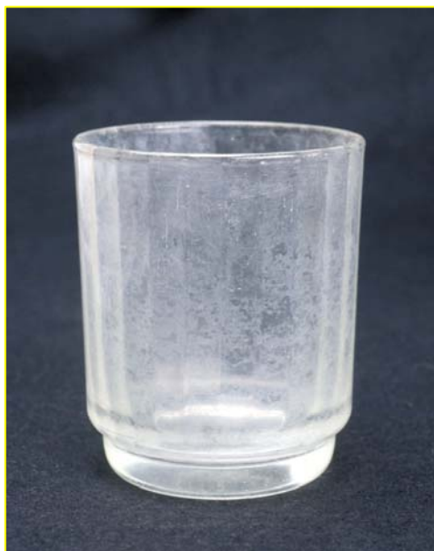
Figure 8. Modern juice glass after approximately five years of cleaning in a dishwasher.
