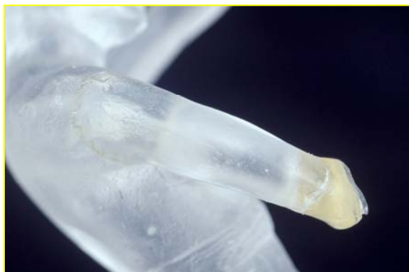
Figure 5. Yellowed adhesive and fill on a glass sculpture (CMOG 59.4.426).
