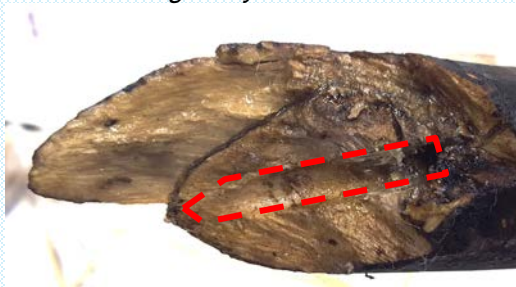
Previous mend during reversal - note diagonally inserted dowel
