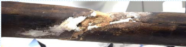
Finished mend with epoxy putty and paper pulp fill material
