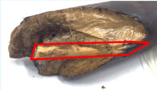
Previous mend during reversal - note diagonally inserted dowel
